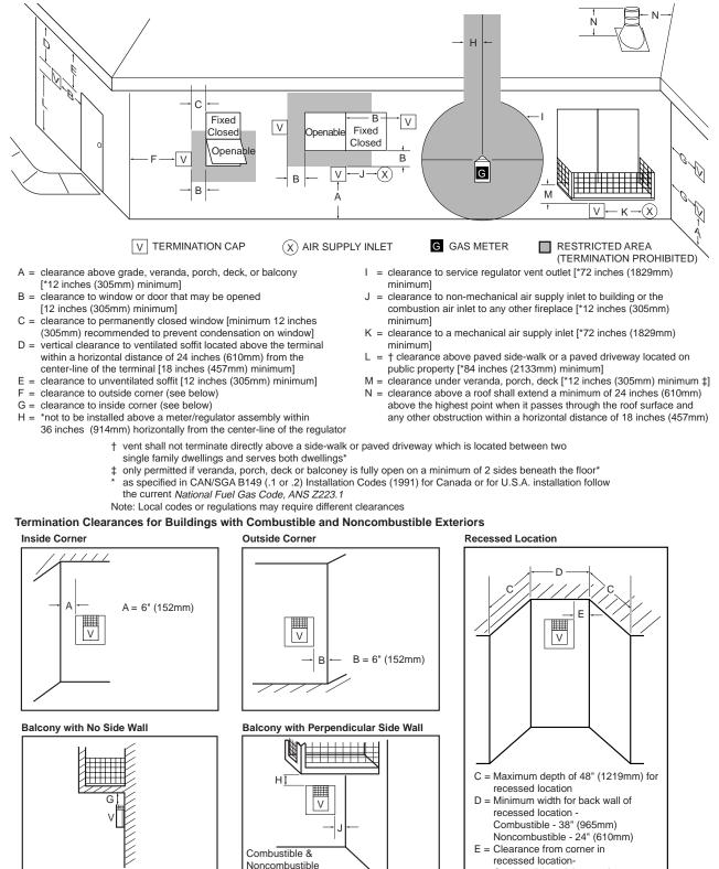
Figure 8 - Minimum Clearances for Vent Terminations
